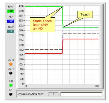
After a positive signal (+24V) at input IN0 the transmitter power is adjusted such that the sensor is in its dynamic range, which is set by **DYN WIN LO** and **DYN WIN HI**.
