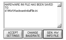
Instruments The baudrate for data transfer through the RS232 interface can be set by means of the SELECT BAUDRATE drop down menu and CHANGE BAUDRATE function field.
