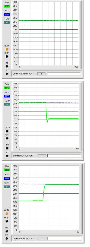
When the current measurement value **RAW** (green line) falls below the switching threshold (red line), the output **OUT0** changes to 0V (error). This is visualised by the **OUT0** LED.
