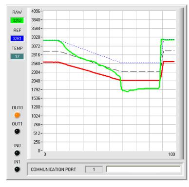
In this example a value of 50 was specified for TT DOWN. This means that downward threshold tracing is performed at a relatively slow speed.
