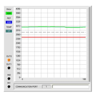
THRESHOLD MODE = LOW: Switching threshold = REF – TOLERANCE Hysteresis threshold = REF - HYSTERESIS
